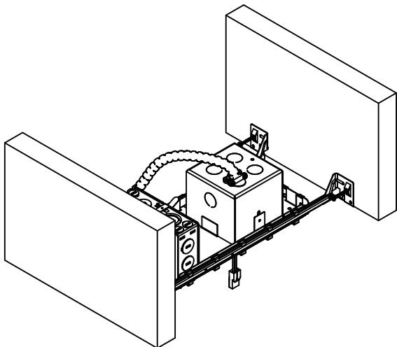
1. Put the Junction Box to the Wood Joist Properly.
