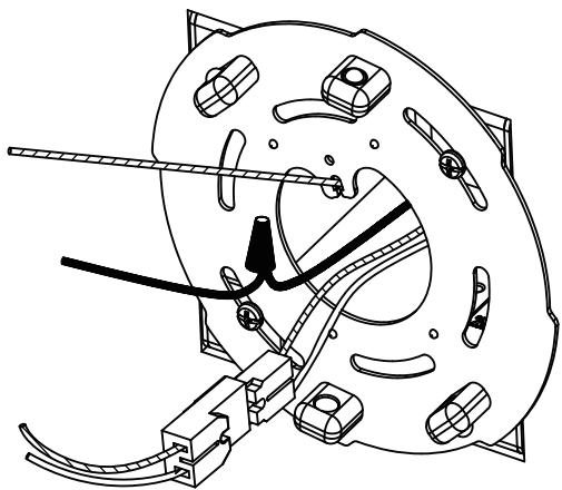
3. Make the wire connections . The green(ground wire) of housing to green of fixture, Female connection of housing to male connection of fixture.
