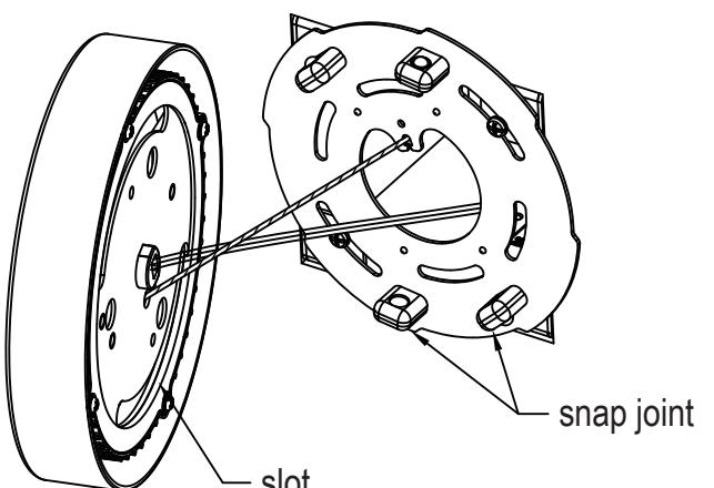
4. Push and feed all wires up into Junction Box as you raise the fixture up into place with right channel.
