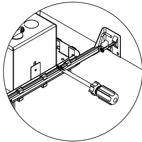
2. Fix the Hanger Bar to Wood Joist with Rivet.
