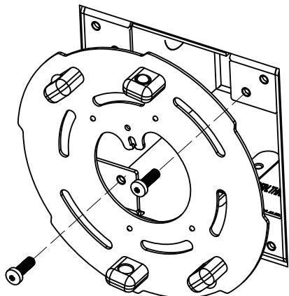
1. To secure installation bracket of fixture to square housing with screws.
