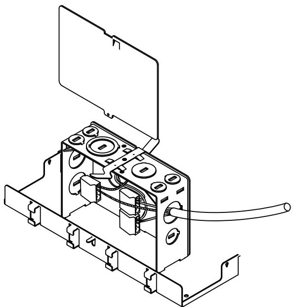
6. Insert cable into the knock-out opening and push the required cable length into the wiring box, the cable will be trapped. Make connection ,Connect white(neutral wire) to white; black(live wire) to black, green(ground wire) to green.
