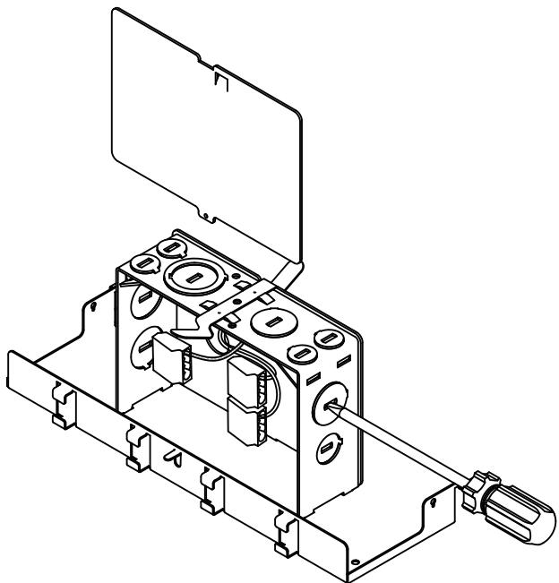
5. Remove wiring box cover. Remove the appropriate knock-out(s) to accommodate the type of electrical supply being used.
